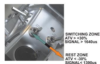
Whenever you turn the device on, it check that the signal from receiver corresponds to the rest position; if the signal is not correct, the LED starts flashing slow for indicating an error and the Kill Switch doesn't activate.
