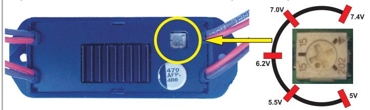
If you want to set a voltage between values indicated or with a precision to one tenth of a volt, you are suggested to use a voltmeter in order to read the output voltage while setting.
